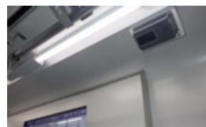
Security camera installed on a Hanshin Electric Railway train
