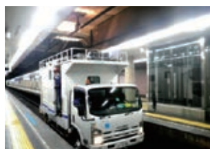
Abrasion measurement by an overhead-wire-inspection vehicle
