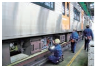
A monthly status and function inspection
