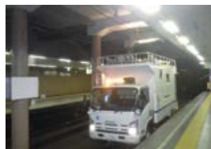
Abrasion measurement by an overhead-wire inspection vehicle
