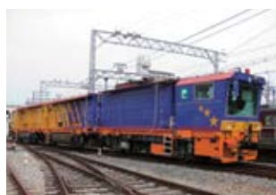
Vehicle for the corrective grinding of rails
