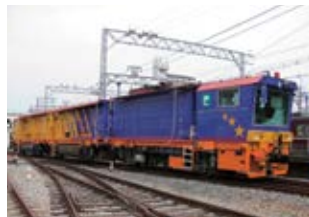
Vehicle for the corrective grinding of rails
