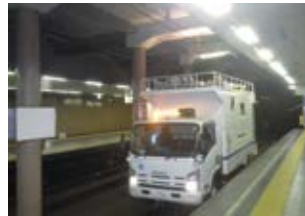
Abrasion measurement by an overhead-wire inspection vehicle
