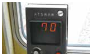
3 ATS indicator in driver's cab
